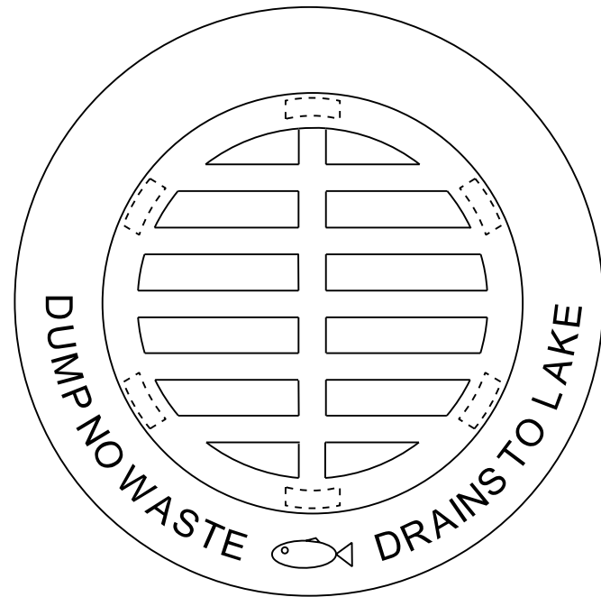
NPDES MESSAGE ON TYPE 8 GRATE
