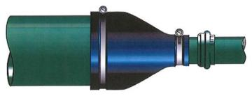
Regardless of style, each end seal shall be manufactured of a minimum 1/8" thick neoprene or synthetic rubber, assuring excellent chemical resistance and resiliency and shall be specifically designed to conform to concentric carrier/casing configuration and to permit movement of the carrier pipe without damage to the seal from backfilling.
