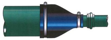
Regardless of style, each end seal shall be manufactured of a minimum 1/8" thick neoprene or synthetic rubber, assuring excellent chemical resistance and resiliency and shall be specifically designed to conform to concentric carrier/casing configuration and to permit movement of the carrier pipe without damage to the seal from backfilling.
