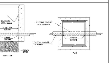
HANDHOLE CONSTRUCTED PER STATE STANDARD 814001.
