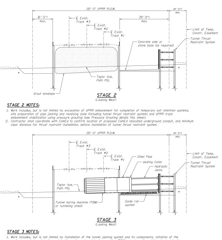
north to south tunnel boring and jacking using a tunnel boring machine (TBM) or a tunneling shield attached to the front steel casing pipe section.
