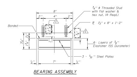
TYPE I ELASTOMERIC EXPANSION BEARING DETAILS
