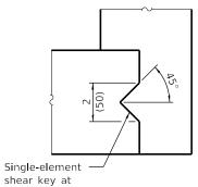
shear key at center of slab
