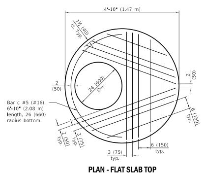
(Showing layout of reinforcement bars and c bars)
