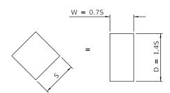
For diamond shaped sign with side S as shown, use required post size for a sign with W = 0.7S and D = 1.4S.
