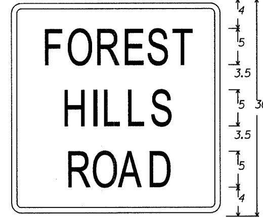
1.9" Radius, 0.8" Border, 0.5" Indent, Black on Orange; [FOREST] C; [HILLS] C; [ROAD] C; Table of letter and object lefts.
