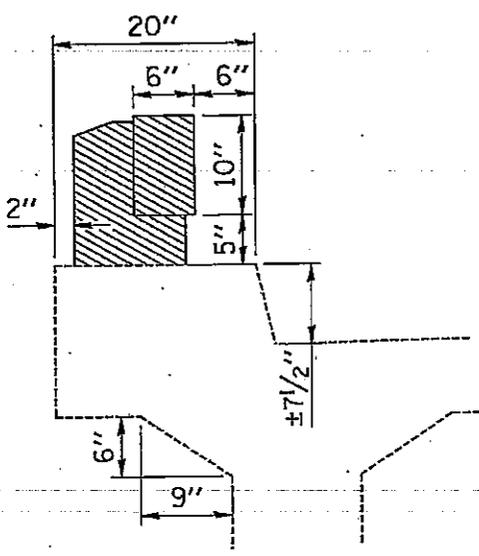
Note: Existing reinforcement bars exposed by handrail concrete removal shall be ground flush with concrete surface and coated with an approved epoxy.
