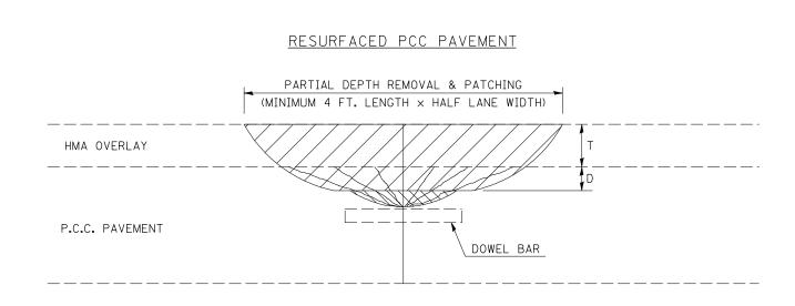
ALL VOLUME OF PARTIAL DEPTH REMOVAL SHALL BE REPLACED WITH HOT-MIX ASPHALT (HMA) AND PAID FOR AT THE CONTRACT UNIT PRICE PER TON FOR PARTIAL DEPTH PATCHING.
