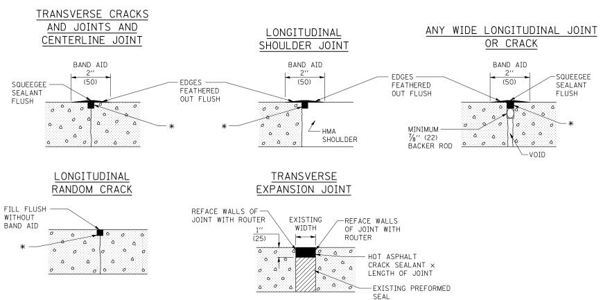
\* HOT ASPHALT CRACK SEALANT
