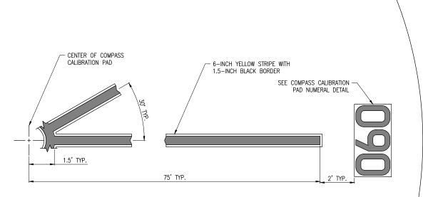
COMPASS CALIBRATION PAD DETAIL NOT TO SCALE
