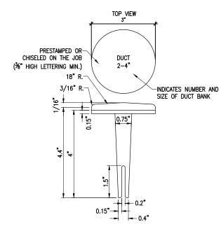
BITUMINOUS PAVEMENT DUCT MARKERS "NOT TO SCALE
