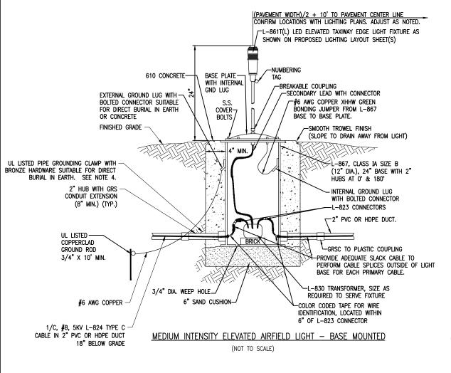
A LIGHT BASE GROUND SHALL BE INSTALLED AT EACH STAKE MOUNTED LIGHT AND FACH TRANSFORMER BASE/LIGHT CAN ASSOCIATED WITH RUNWAY LIGHTS, TAXIWAY LIGHTS, RUNWAY DISTANCE REMAINING SIGNS. AND LIGHTED RUNWAY/TAXI GUIDANCE SIGNS. THE LIGHT BASE GROUND SHALL BE A #6 AWG BARE COPPER CONDUCTOR CONNECTED TO THE GROUND LUG ON THE RESPECTIVE L-867 TRANSFORMER BASE/LIGHT CAN OR MOUNTING STAKE AND A 3/4-INCH DIAMETER BY 10-FEET LONG (MINIMUM) UL LISTED COPPER CLAD GROUND ROD.
