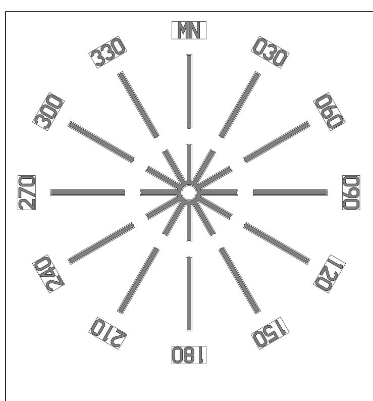
COMPASS CALIBRATION PAD MARKINGS NOT TO SCALE
