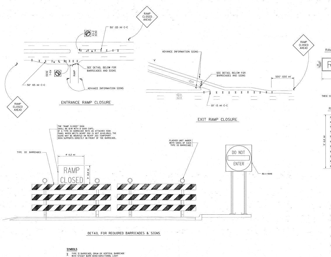
TYPE III BARRICADE WITH FLASHING LIGHT
