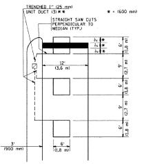
\*\* UNIT DUCT IS TO BE SHOWN ON PLAN SHEETS BUT SHALL NOT BE INCLUDED IN THE PAY ITEMS. NOTE: DUAL LEFT TURNS NOT SHOWN REFER TO PLAN SHEET FOR DETECTOR LOOP REPLACEMENT
