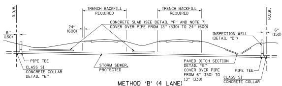
STORM SEWER LESS THAN 2' (600 mm) BELOW DITCH FLOW LINE AND STORM SEWERS CROSSING UNDER PAVEMENTS AND PAVED DITCHES
