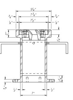
Drill and tap 8 holes for <sup>1</sup>2"-13 bolts on an 8<sup>3</sup>4" \$ bolt circle, (2 blind holes are  $1^{l_4}$ " deep, 6 thru holes)
