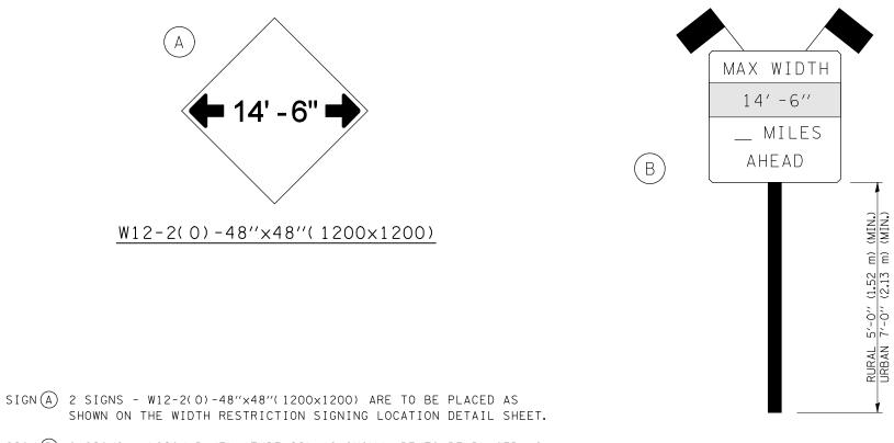
SIGN B 2 SIGNS - (SIGN PANEL, TYPE II) AS SHOWN ARE TO BE PLACED AS SHOWN ON THE WIDTH RESTRICTION SIGNING LOCATION DETAIL SHEET.
