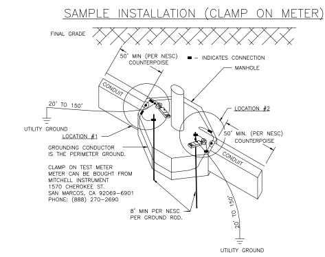
OBSERVE ALL SAFETY REQUIREMENTS AND THEN REMOVE COVERING ON THE GROUND CONDUCTOR IF PRESENT AND PROVIDE SUFFICIENT ROOM FOR THE MODEL 3710/3730 JAWS, WHICH MUST BE ABLE TO CLOSE EASILY AROUND THE CONDUCTOR. THE JAWS CAN BE PLACED AROUND THE GROUND ROD ITSELF.
