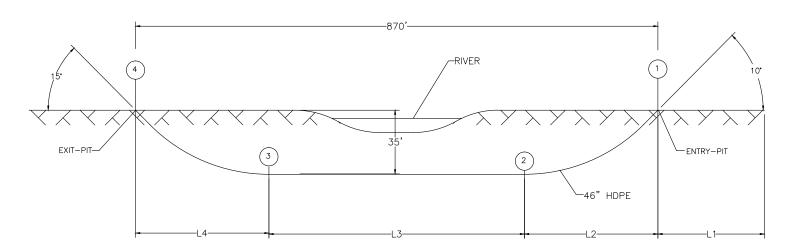
TYPICAL RIVER CROSSING, ASSUME THE HDPE PIPE IS 35' DEEP AND APPROXIMATELY 870' LONG WITH A 10 DEG. ENTRY ANGLE AND A 15 DEG. EXIT ANGLE. ACTUAL PULL BACK FORCE WILL VARY DEPENDING ON HACKREAMER SIZE SELECTION, AND USE; BORE HOLE STAYING OPEN; SOIL CONDITIONS; LUBRICATION WITH BENTONITE, DRILLER EXPERTISE, AND OTHER APPLICATION CIRCUMSTANCES.
