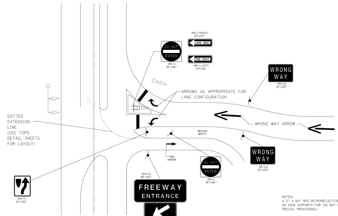
A 2" × 60" RED RETROREFLECTIVE SIGN SUPPORT PANEL SHOULD BE PLACED ON SIGN SUPPORTS FOR 'DO NOT ENTER' AND 'WRONG WAY' SIGNS. (SEE
