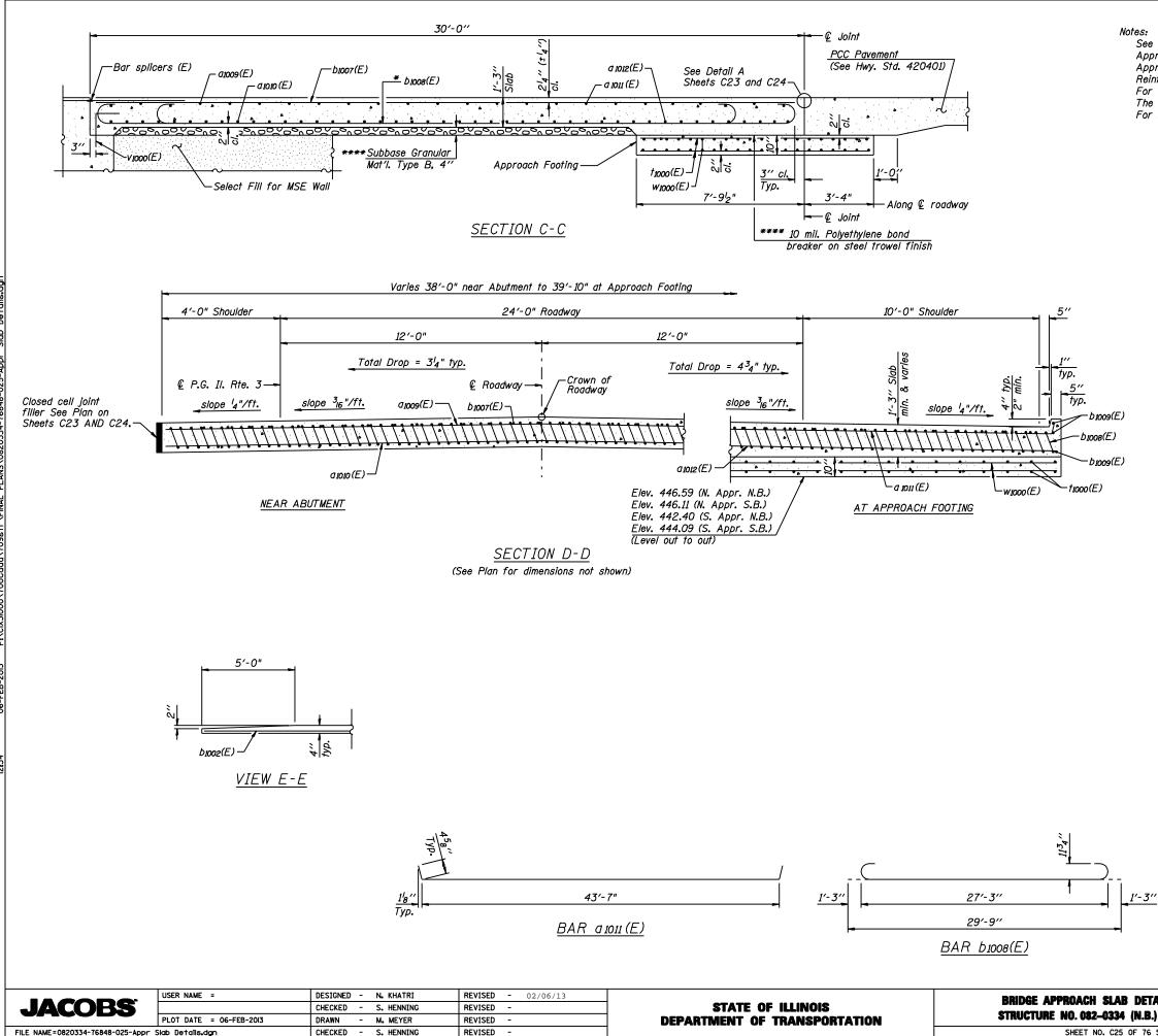
See Sheets C23 and C24 for Detail A. Approach Slab shall be paid for as Concrete Superstructure. Approach Footing concrete shall be paid for as Concrete Structures. Reinforcement shall be paid for as Reinforcement Bars, Epoxy Coated. For v1000(E) bar details, see Sheets C36 thru C43. The approach footing maximum applied service bearing pressure (Qmax) = 2.0 ksf. For bar splicer details, see sheet C50.
