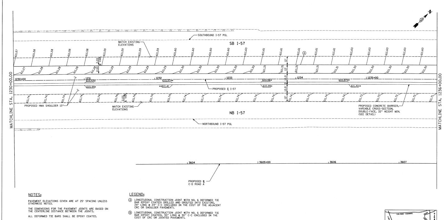
CONTRACTION JOINTS (UNDOWELED-SAWED OR GROOVED) SHALL BE PROVIDED ACROSS ALL PCC SHOULDERS. JOINT SPACING SHALL BE 20' C-C UNLESS OTHERWISE NOTED PER STANDARD 483001.
