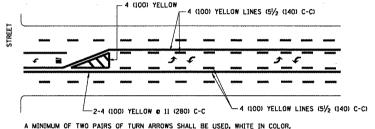
A MINIMUM OF TWO PAIRS OF TURN ARROWS SHALL BE USED, WHITE IN COLOR, ADDITIONAL PAIRS SHALL BE PLACED AT 200' (60 m) TO 300' (90 m) INTERVALS.
