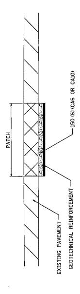
THE CA 6 OR CA 10 SHALL BE COMPACTED IN A MANNER APPROVED BY THE ENGINEER. IF THE MOISTURE CONTENT OF THE MATERIAL IS SUCH THAT COMPACTION SATISFACTORY TO THE ENGINEER CANNOT BE OBTAINED, SUFFICIENT WATER SHALL BE ADDED SO THAT SATISFACTORY COMPACTION CAN BE OBTAINED.
