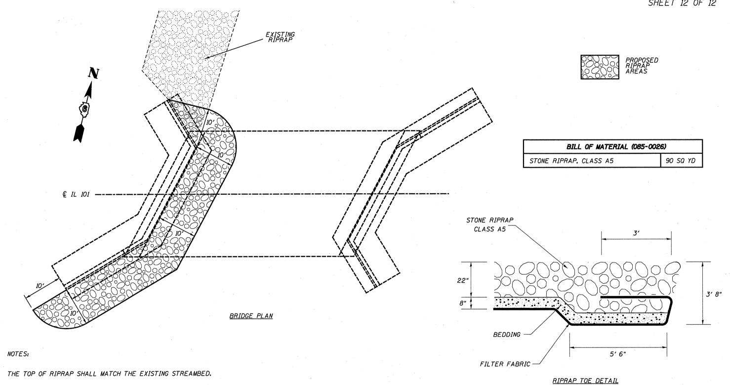
THE RIPRAP TOE DETAIL SHALL BE USED AROUND ALL EDGES OF THE RIPRAP AREA THAT ARE NOT ADJACENT TO THE EXISTING BRIDGE.
