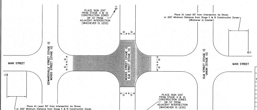
CONSTRUCTION ZONES II & III (CLOSED TO VEHICULAR TRAFFIC) • TYPE III BARRICADE WITH FLASHING LIGHTS
