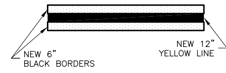
TAXIWAY CENTERLINE CONTINUOUS N.T.S.
