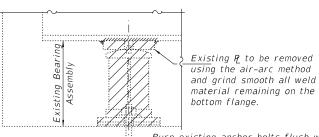
Burn existing anchor bolts flush with existing concrete surface. Grind existing anchor bolt smooth and seal with epoxy.
