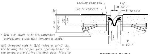
SECTION THRU WELDED RAIL JOINT
