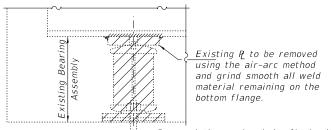
Burn existing anchor bolts flush with existing concrete surface. Grind existing anchor bolt smooth and seal with epoxy.
