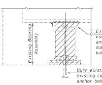
Existing P to be removed using the air-arc method and grind smooth all weld material remaining on the bottom flange.
