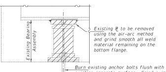
existing concrete surface. Grind existing anchor bolt smooth and seal with epoxy.
