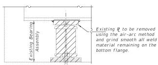
Burn existing anchor bolts flush with existing concrete surface. Grind existing anchor bolt smooth and seal with epoxy.
