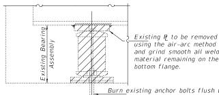
using the air-arc method and grind smooth all weld material remaining on the bottom flange.
