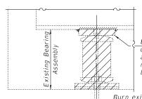
Existing P to be removed using the air-arc method and grind smooth all weld material remaining on the bottom flange.
