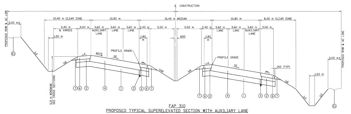
NOTE: STA 39+108.322 TO STA 39+195.000 SBL 4.0% STA 39+195.000 TO STA 39+260.000 SBL SE TRANSITION STA 39+260.000 TO STA 39+410.000 SBL FULL SE (5.5%) CURVE NO 3 (RIGHT)
