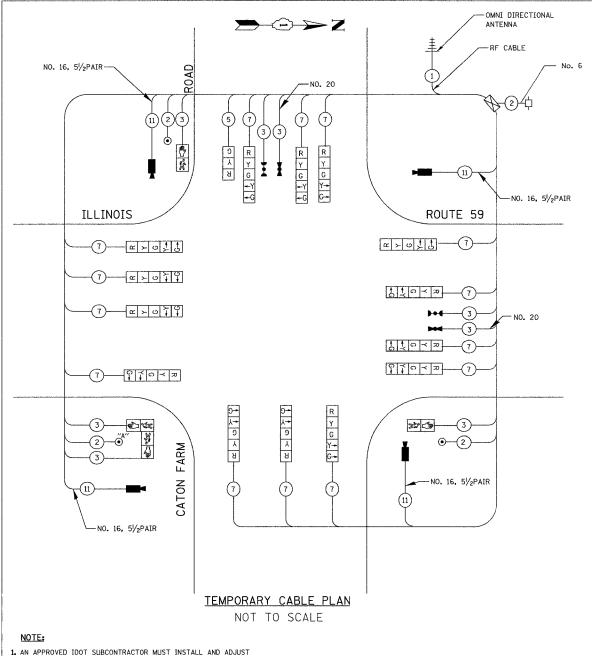
AN APPROVED IDOT SUBCONTRACTOR MUST INSTALL AND ADJUST VIDEO VEHICLE DETECTION SYSTEM AS REQUIRED BY STAGE/ PHASE CHANGES. ADJUSTMENT WILL BE REQUIRED BETWEEN PRIMARY AND SECONDARY.
