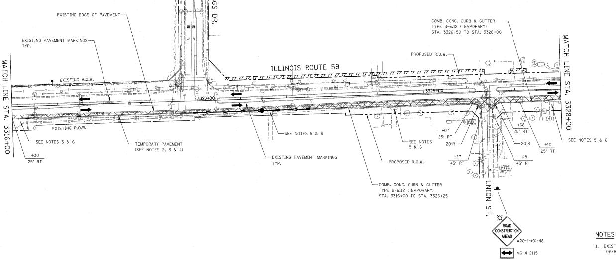
FOR TEMPORARY PAVEMENT CONSTRUCTION USE HIGHWAY STANDARDS NO. 701326 & 701701
