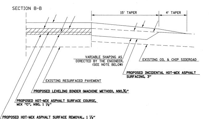
IF EXISTING SUB-BASE IS INADEQUATE, AS DETERMINED BY THE ENGINEER, THE SIDEROADS SHALL BE CORED OUT AND AGGREGATE SUB-BASE, TYPE B SHALL BE PLACE FOR BASE. THE COST OF CORING OUT THE SIDEROAD SHALL BE INCLUDED IN THE COST OF THE AGGREGATE BASE COURSE. IF EXISTING SUB-BASE IS DETERMINED TO BE ADEQUATE, THE AGGREGATGE BASE COURSE SHALL BE DELETED AND THE PREPARATION OF THE BASE SHALL BE CONSTRUCTED ACCORDING TO ARTICLE 406.09.
