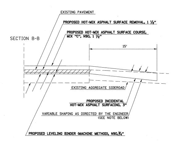
IF EXISTING SUB-BASE IS INADEQUATE, AS DETERMINED BY THE ENGINEER, THE SIDEROADS SHALL BE CORED OUT AND AGGREGATE SUB-BASE, TYPE B SHALL BE PLACE FOR BASE. THE COST OF CORING OUT THE SIDEROAD SHALL BE INCLUDED IN THE COST OF THE AGGREGATE BASE COURSE. IF EXISTING SUB-BASE IS DETERMINED TO BE ADEQUATE, THE AGGREGATGE BASE COURSE SHALL BE DELETED AND THE PREPARATION OF THE BASE SHALL BE CONSTRUCTED ACCORDING TO ARTICLE 406.09.
