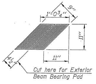
The bearing seat surfaces shall be adjusted by shimming to assure firm and even bearing prior to placement of grout. Two  $^{l}_{8}$ " fabric adjusting shims of the dimensions of the Exterior Bearing Pad shown shall be provided for each bearing 132 Required).
