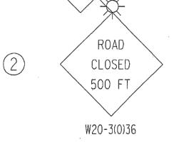
Post mounted sign with 18" x 18" (Minimum) orange flag and Type A Flashing Light.
