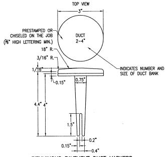
BITUMINOUS PAVEMENT DUCT MARKERS "NOT TO SCALE"
