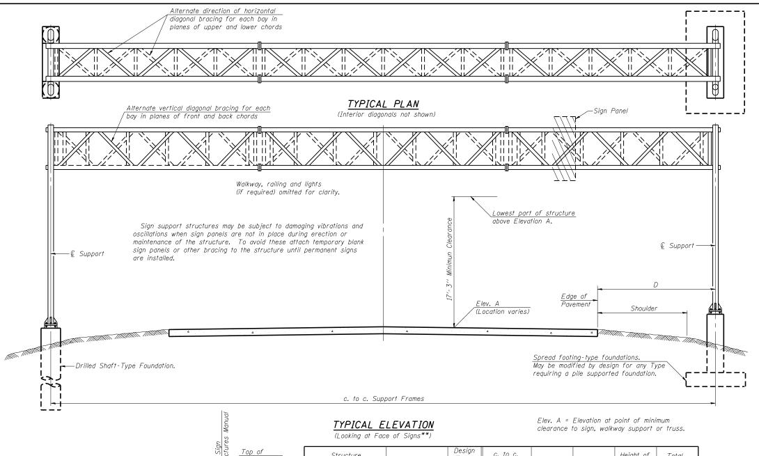
End Support 30 p.s.f. SN-03 (See Sign Structures 10 D.S.1 SN-03 Manual for max. sign areas) SN-03 SN-03 34'-0'', may Type III-A SN-03 Maximum Lenath c. to c. Support Frames (See Sign Structures Manual)
