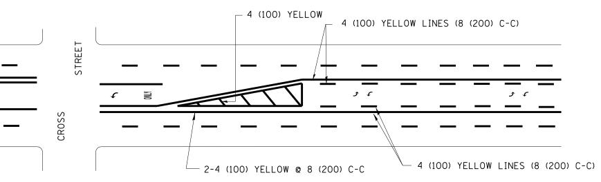
A MINIMUM OF TWO PAIRS OF TURN ARROWS SHALL BE USED, WHITE IN COLOR. ADDITIONAL PAIRS SHALL BE PLACED AT 200' (60 m) TO 300' (90 m) INTERVALS.
