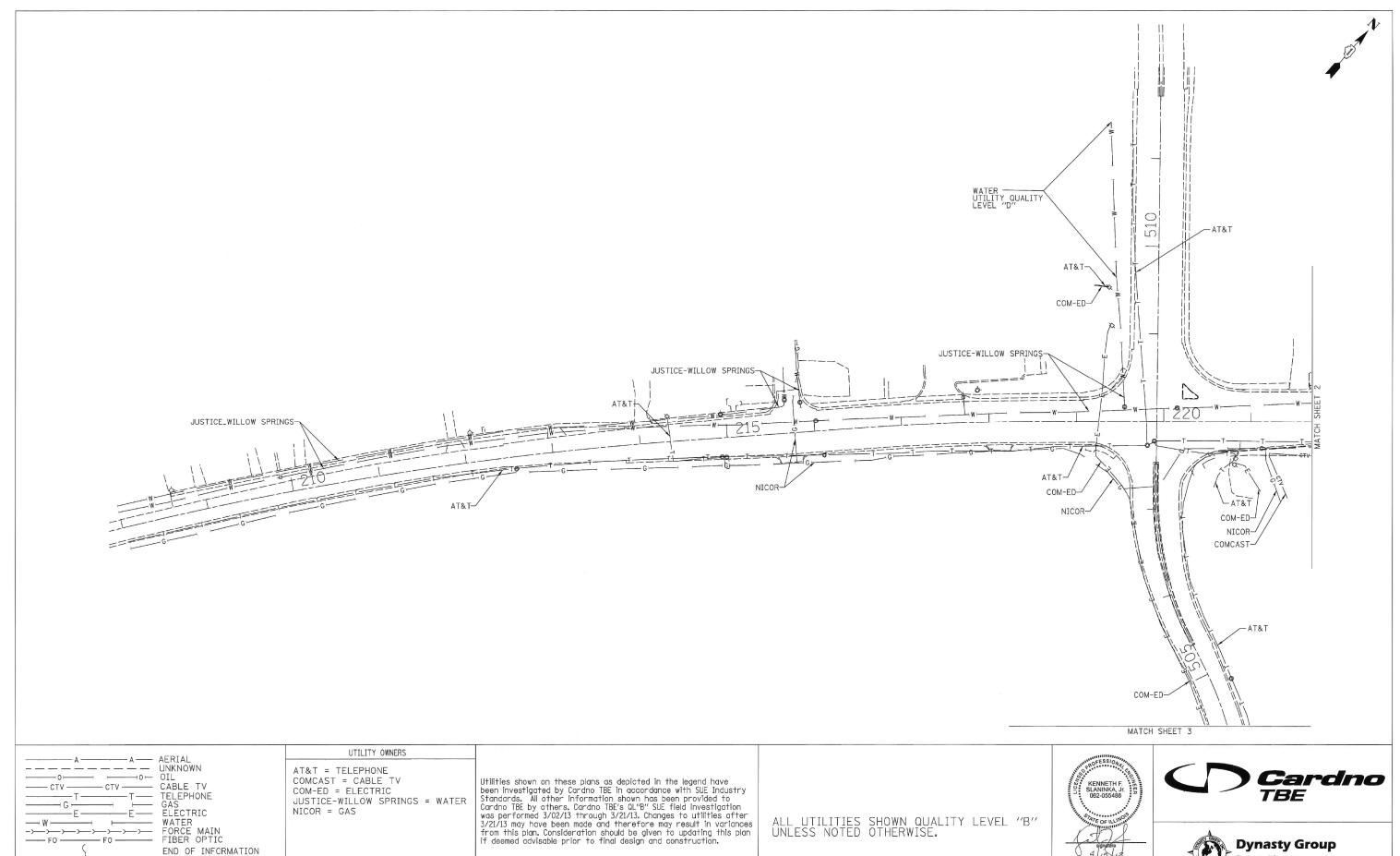
Utility Quality Level "A": Visually Verified Test Hole Utility Quality Level "B": Designating/non Visually Verified Test Hole Utility Quality Level "C": Research with Survey Utility Quality Level "D" : Records Research
