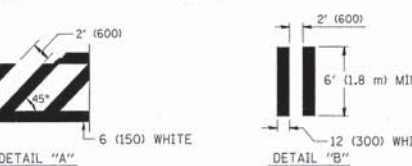
TYPICAL CROSSWALK MARKING
