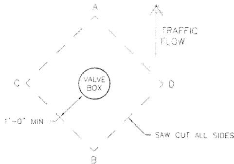
1. WATER VALVE BOX SHALL BE ADJUSTED AFTER PAVING IS COMPLETED.
