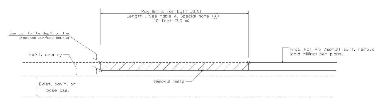
CASE 4: SINGLE LIFT OVERLAY WITH EQUIVALENT DEPTH
