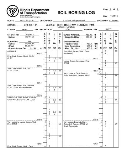
The Unconfined Compressive Strength (UCS) Failure Mode is indicated by (B-Bulge, S-Shear, P-Penetrometer)
