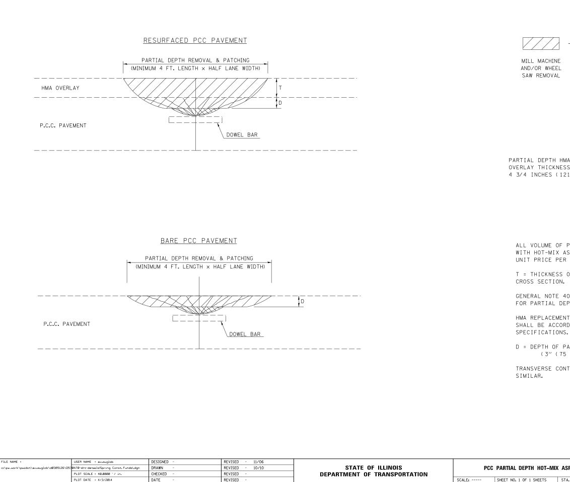
AIR EQUIPMENT OR MECHANICAL SWEEPER REMOVAL OF LOOSE AND/OR UNSOUND CONCRETE
