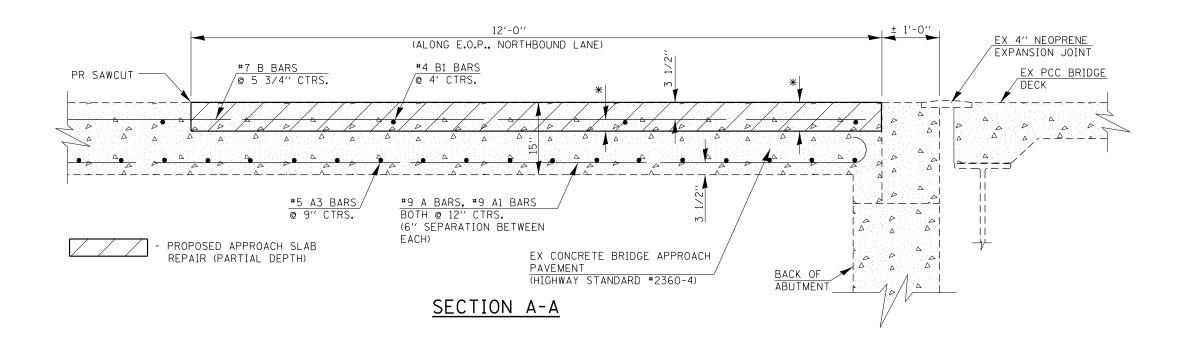
\* — THE DEPTH OF PROPOSED SLAB REPAIR SHALL BE 1" MINIMUM BELOW THE TOP REINFORCEMENT MATTING. PROPOSED SLAB REPAIR SHALL NOT EXCEED 6" MAXIMUM.
