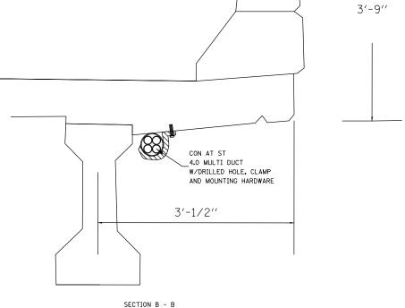
DIMENSIONS REQUIRE FIELD VERIFICATION PRIOR TO STRUCTURE DRILLING, CLAMP FABRICATION AND FASTENING HARDWARE SELECTION
