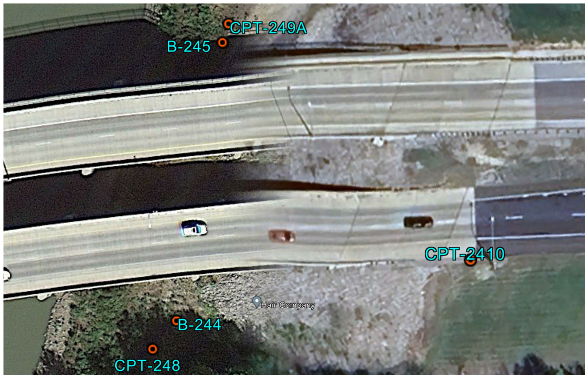
Figure 5: Boring and CPT locations for the 2024 subsurface investigation on the east side of the river.
