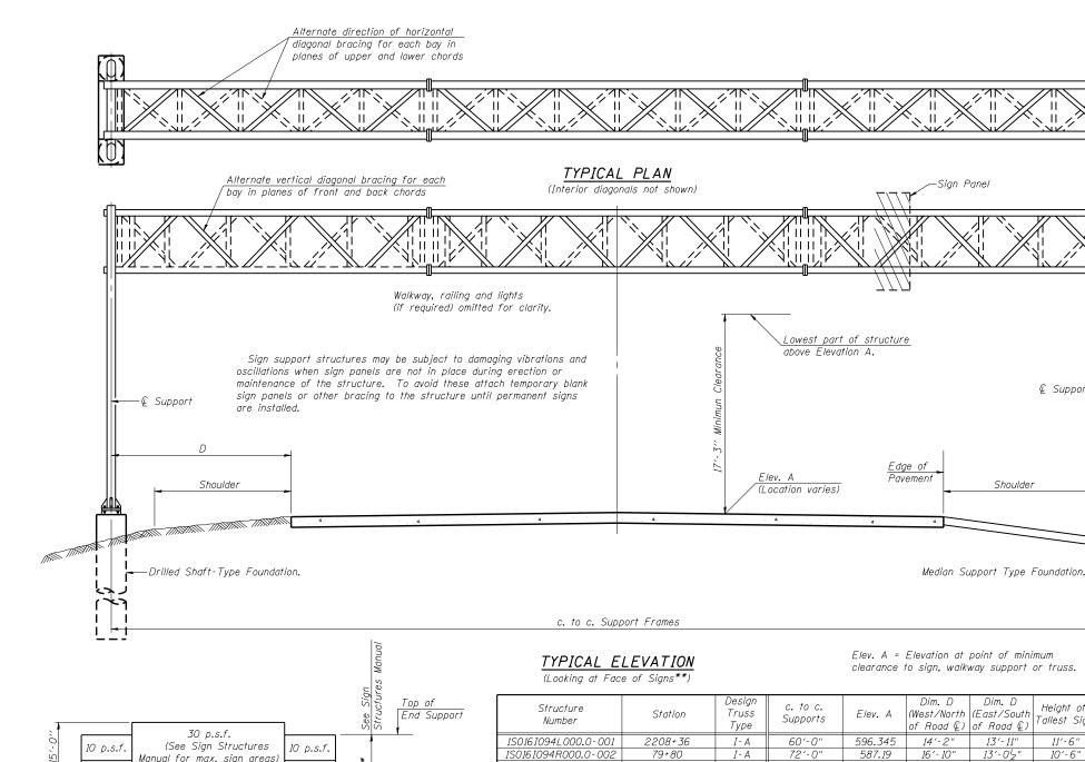
Elev. A = Elevation at point of minimum clearance to sign, walkway support or truss.
