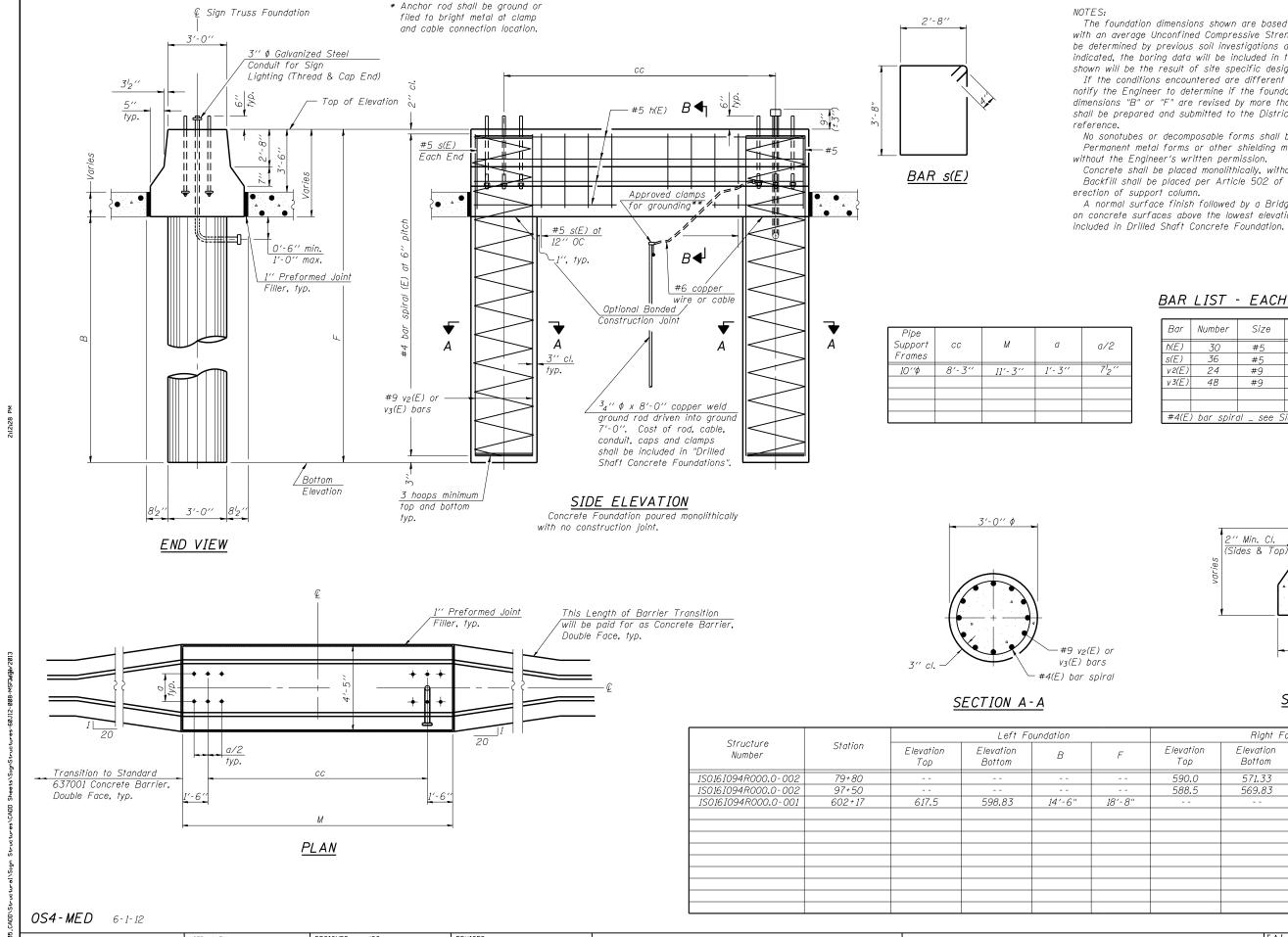
The foundation dimensions shown are based on the presence of mostly cohesive soils with an average Unconfined Compressive Strength (Qu) of at least 1.25 tsf, which must be determined by previous soil investigations at the jobsite. When other conditions are indicated, the boring data will be included in the plans and the foundation dimensions shown will be the result of site specific designs.
