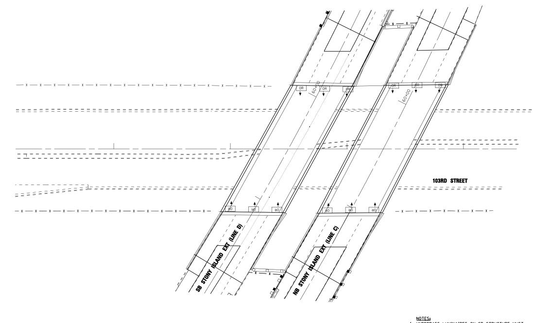
NOTES: 1. UNDERPASS LUMINAIRES ON SB STRUCTURE MUST REMAIN IN OPERATION DURING STAGE I CONSTRUCTION. PROPOSED UNDERPASS LUMINAIRES ON NB STRUCTURE MUST BE ACTIVATED AT THE COMMENCEMENT OF STAGE II CONSTRUCTION.
