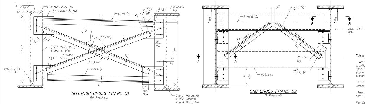
All cross frames between girders shall be installed with erection pins and bolts in accordance with the erection plan approved by the Engineer. Individual cross frames at supports may be temporarily disconnected to install bearing anchor rods.
