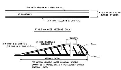
DIAGONAL LINE SPACING: 50' (15 m) C-C (LESS THAN 30MPH (50 km/h))
