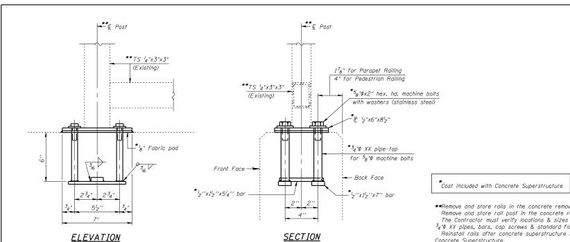
RAIL POST REMOVAL & REPLACEMENT DETAILS FOR PARAPET RAILING & PEDESTRIAN RAILING \*\*Remove and store rails in the concrete removal area prior to concrete removal.
